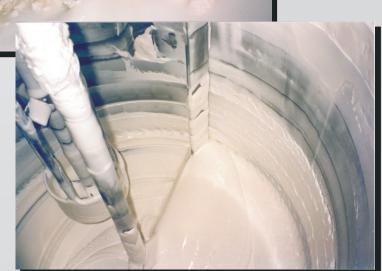
Mandatory for a homogeneous and reproducible batch emulsifying process is a perfect mixing of the contents in the vessel in combination with a system that applies sufficient shear energy to delay the dispersed droplets from recombining until the emulsifier has coated their surface.
